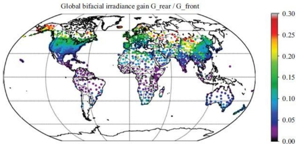
Figure 3.16: Results of modelling for the bifacial rear-irradiance gain for a fixed latitude tilted system ( $h=1$  m,  $r$  is based on latitude and tilt) [33]
