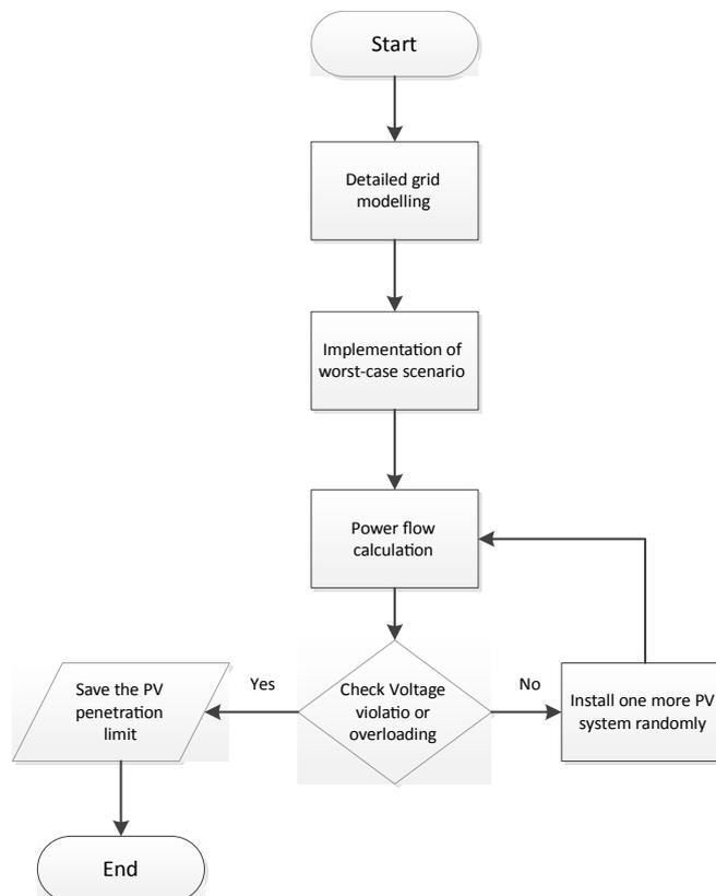
**Figure 4.3: Simplified algorithm to estimate the grid hosting capacity considering voltage and overloading constraints**
