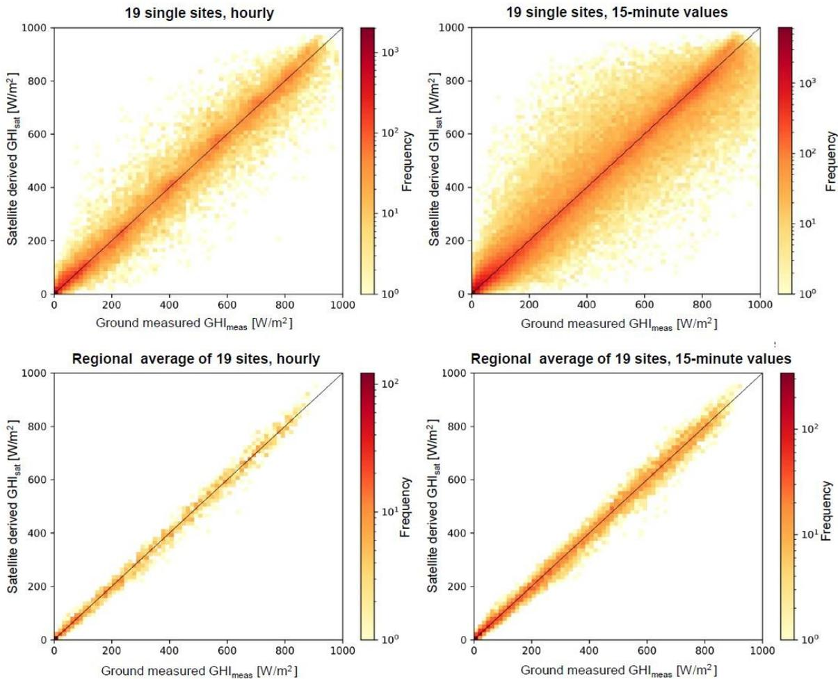
**Figure 3.21: 2d Histogram of satellite derived versus ground measured irradiance with corresponding RMSE values**
