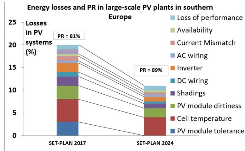
Figure 3.9: Energy losses and performance ratio before and after SERENDI-PV for large-scale PV plants in southern Europe
