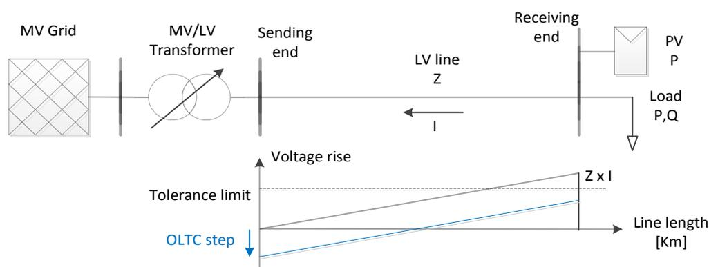
Figure 4.7: Schematic illustration of the voltage rise considering OLTC control
