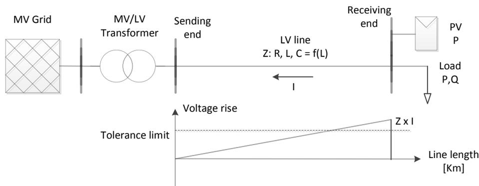
**Figure 4.2: Schematic illustration of the voltage rise at receiving-end considering high PV feed-in**
