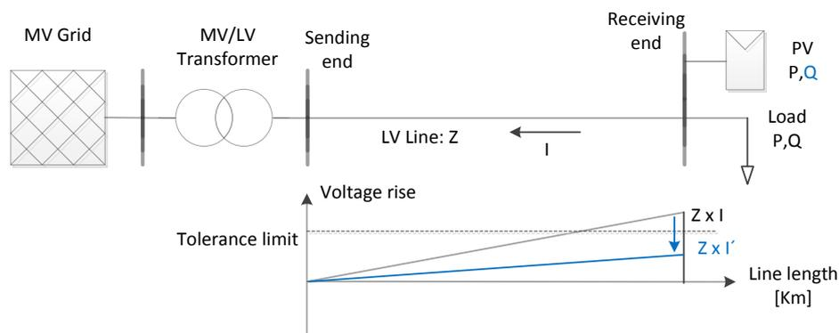
Figure 4.5: Schematic illustration of the voltage rise considering reactive power provision of PV
