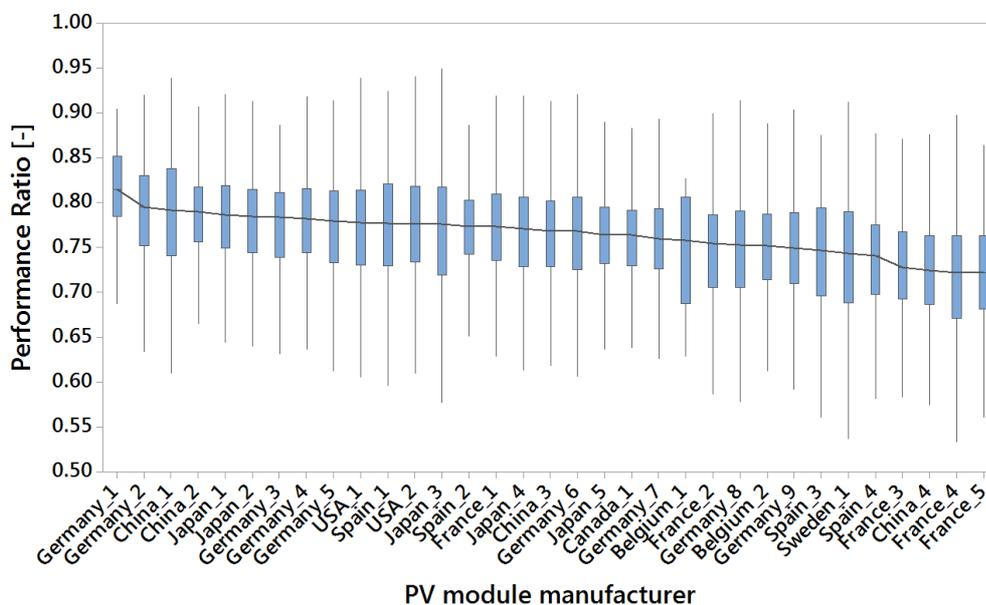
**Figure 3.8: Boxplot representing the yearly PR for the PV modules that equip at least 100 PV systems (excluding thin-film technologies). We observe that there is a difference in the median value of PR of some 6% between the best performer and the worst performer**
