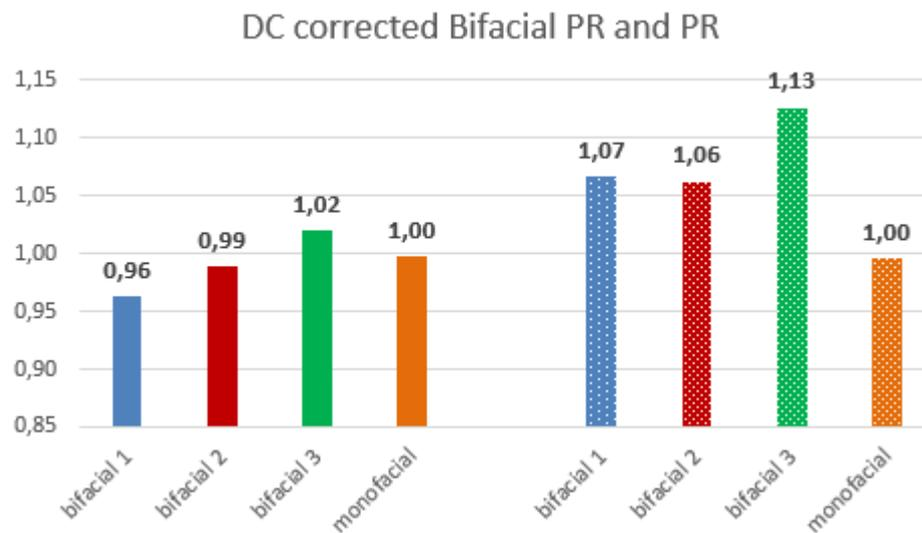
Figure 3.12: Examples of DC temperature corrected bifacial PR (left) and DC temperature corrected PR (right) for 4 string PV systems [Source CEA internal measurements]
