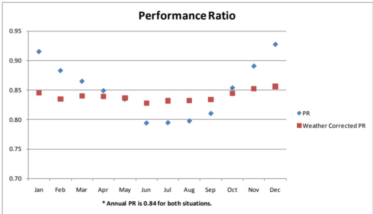
Figure 3.11: Results of modelling of uncorrected PR and weather corrected PR [22]
