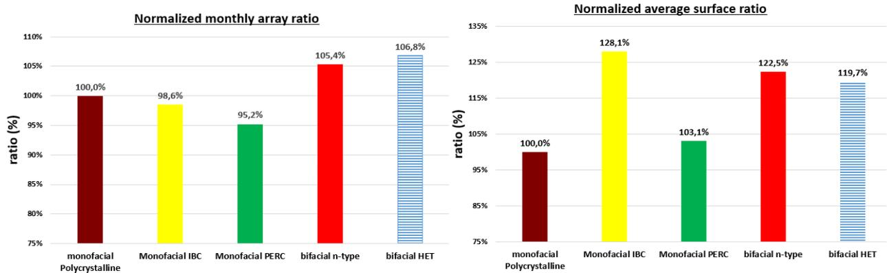
Figure 3.15: Examples of normalized DC PR (left) and DC SuR (right) for 5 string PV systems [source CEA]
