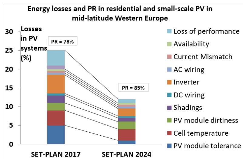
Figure 3.10: Energy losses and performance ratio before and after SERENDI-PV for Small-scale and residential PV installations in mid-latitude western Europe
