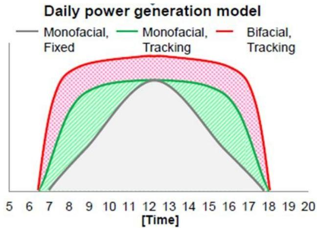
Figure 3.18: Schematic of tracking gains with monofacial and bifacial modules
