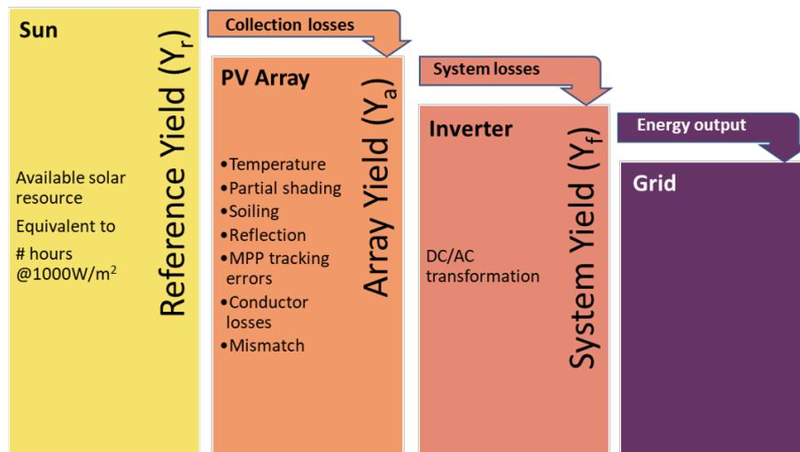
Figure 3.1: Energy yield flow evaluation scheme for grid-connected PV systems
