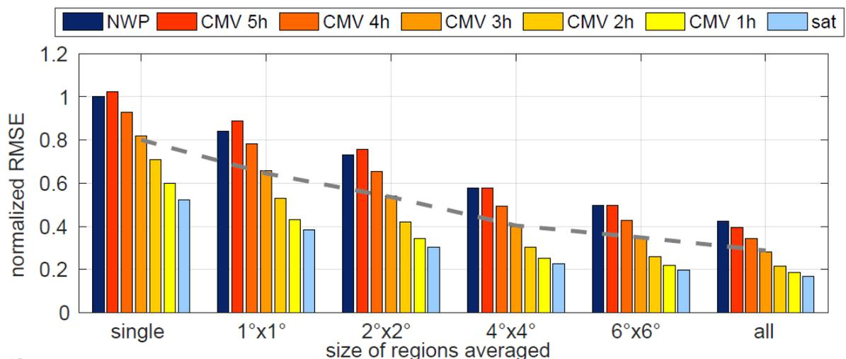
Figure 3.23: RMSE of hourly irradiance predictions for averages for different regions size, normalized to NWP single site forecast errors. The predictions are based on cloud motion vectors from satellite data (‘CMV’) for different forecast horizons, on numerical weather predictions (‘NWP’) for day-ahead forecasts. They are compared to satellite derive irradiance values (‘sat’). Dataset: 217 irradiance measurement stations in Germany, Jan 2012– December 2013. Source: [48]
