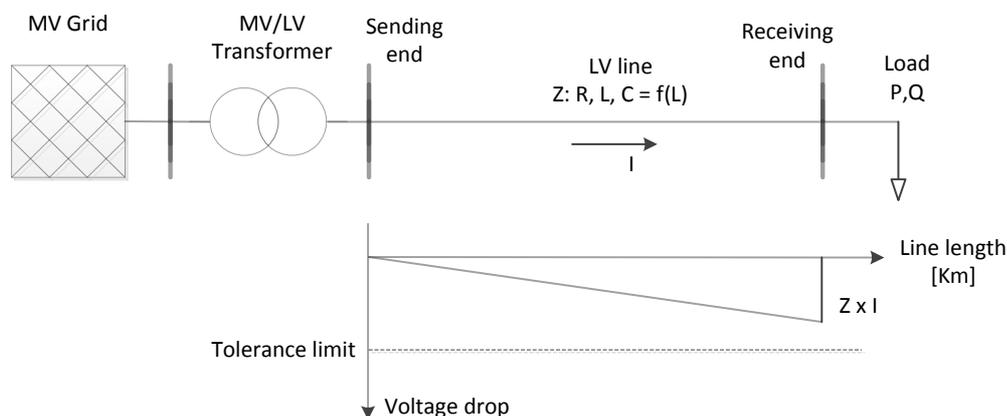
**Figure 4.1: Schematic illustration of the voltage at receiving end considering a simple line**
