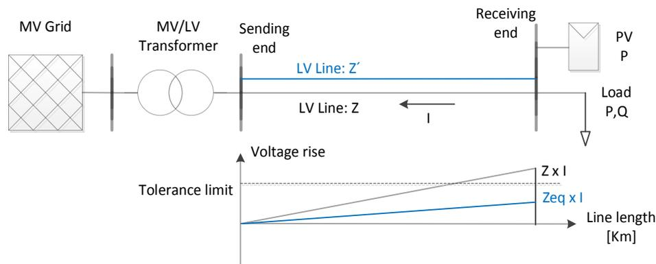
Figure 4.4: Schematic illustration of the voltage rise considering adding a parallel line
